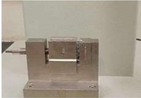
Fig vii. The sample piece broken inside of the holder.
