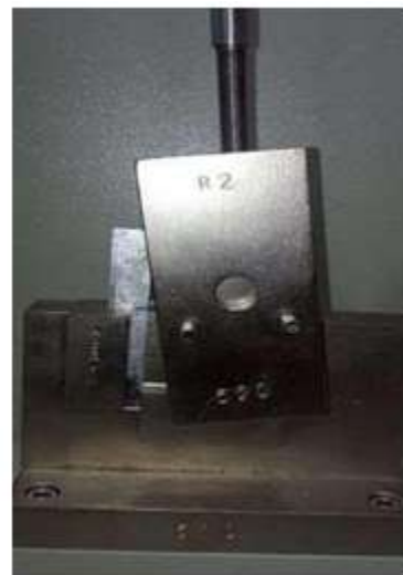
Fig vi. Notched specimen set up in the holder.
