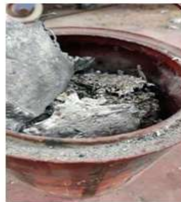
Fig iv. Slag formed during the melting process.
