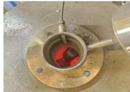
Fig iii. Melting the aluminium ingots in high temperature crucible.
