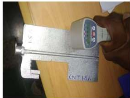
Fig viii. BarcolImpressor being used to test the hardness.
