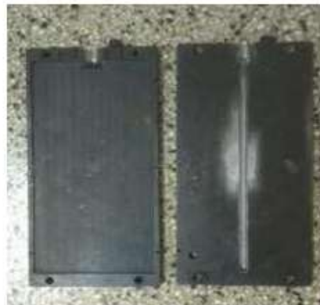
Fig i: Mild Steel Die used to make the specimen
